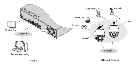
DirectIP™ NVR makes it easy to use cameras without extra network configurations.
