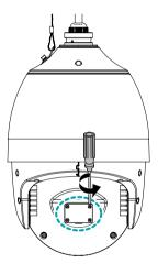
Insert a SD memory card into the SD memory card slot with the 'micro SD' print facing upward.
